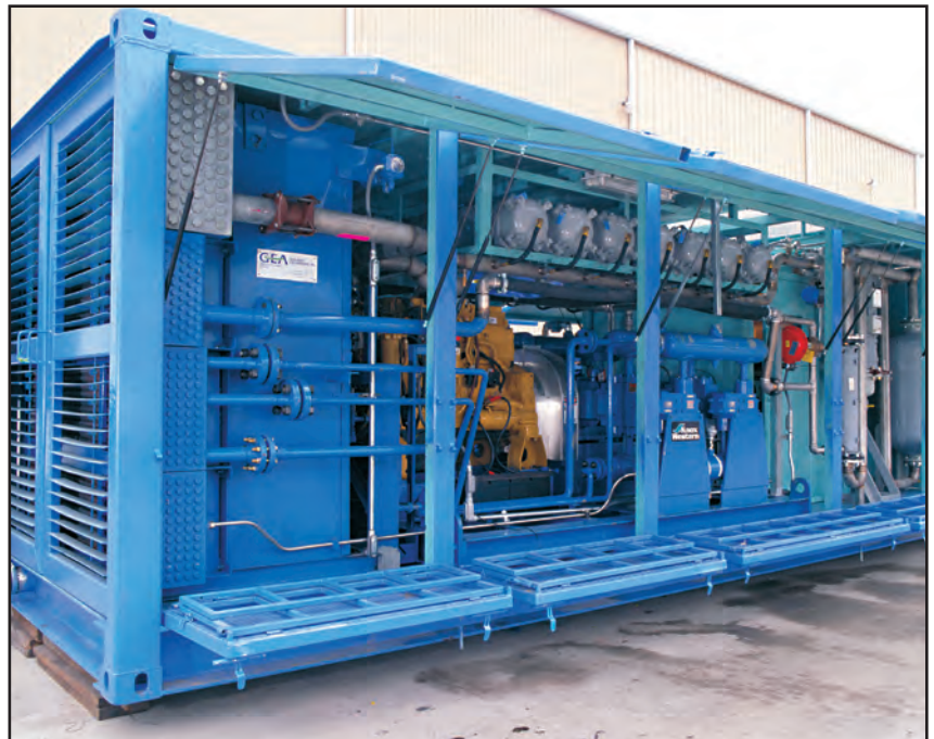
■ Containerized diesel-driven booster compressor and nitrogen unit.
