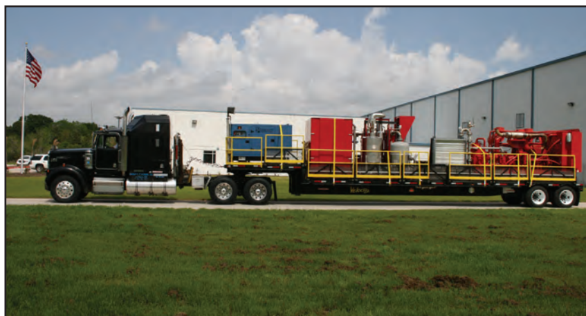
■ Trailer-mounted feed compressor, nitrogen unit and generator.
